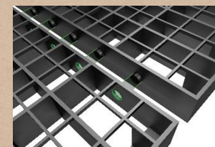
Detail of lateral locks between grids
